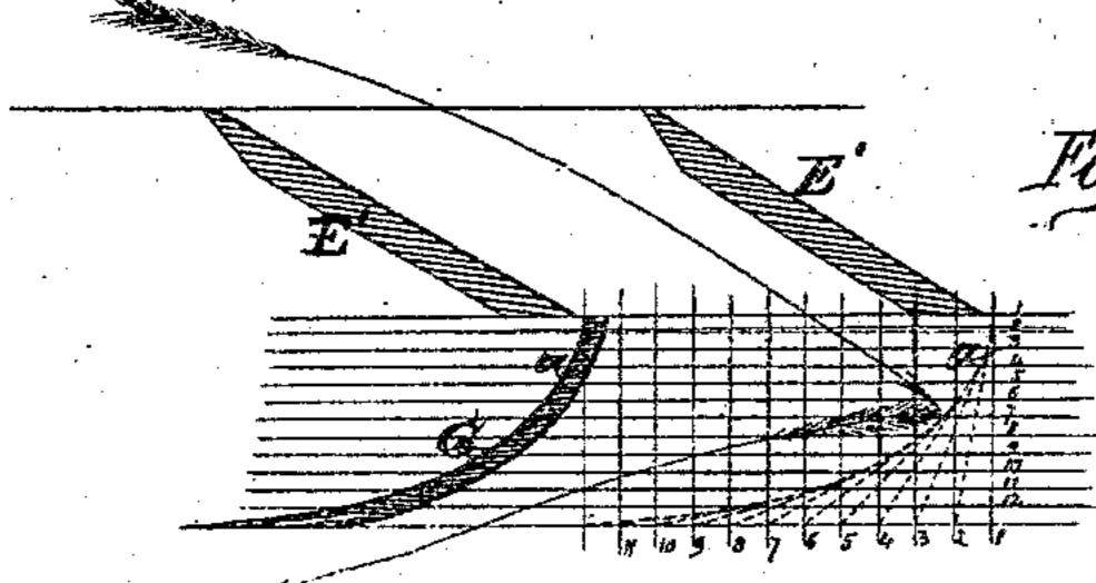
Fig 2. Section shewing method of constructing buckets & shoots.
