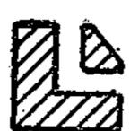
There would then be a slot or channel on two sides, to receive the ends of the weather boarding. This channel is clear from top to bottom. The screw is in the corner. I then make the door and window frames in the ordinary manner and cut a channel down the sides, and at top and bottom, to
